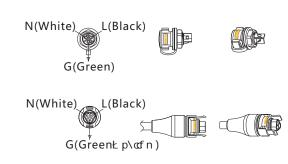
Step4 Plug the AC output line to main AC cable;
