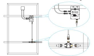
**Step2** Connect the two DC terminal of the PV to the inverter, positive to positive, negative to negative. Show below:
